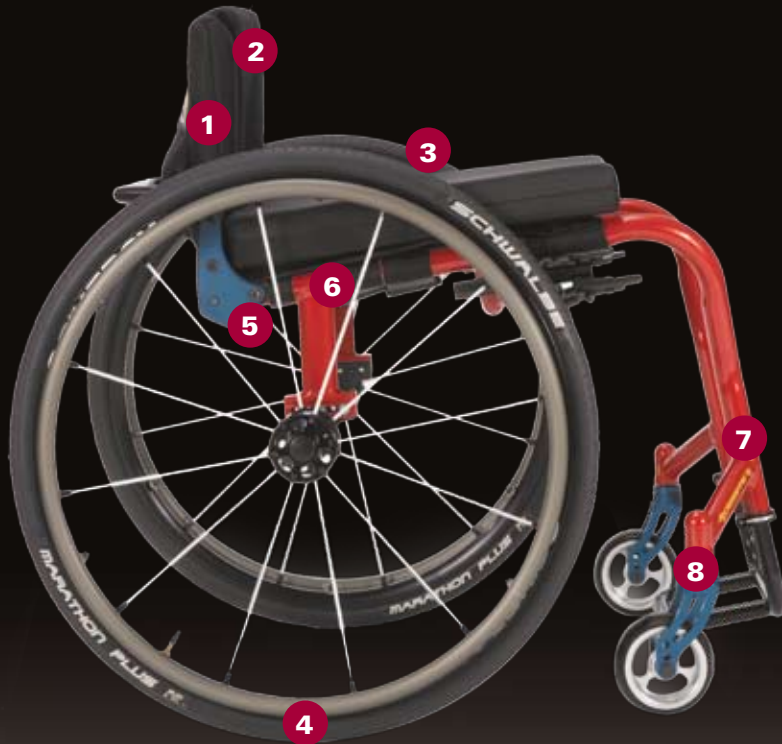
5 The back angle is adjusted simply by loosening a button-head screw and rotating an adjustment square located on the inside of this back bracket.
