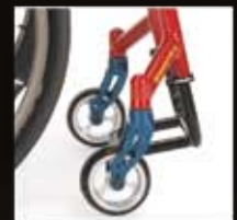
8 Each custom frame is built to accommodate a short front fork to reduce overall caster trail and keep the user's center-of-gravity low to the ground for improved balance.
