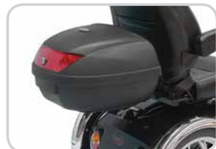
Rear storage pod
