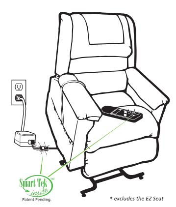
If both LED lights are off, the user should first check that the chair is plugged into an electrical outlet, that the fuse or breaker for that outlet is properly working, and that all other connections are plugged together properly.
