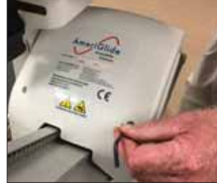
INSERT ALLEN WRENCH TO LOOSEN DRIVE UNIT SIDE COVERS
