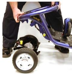
Figure 18. Lifting the Frame
