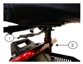
Figure 8. Seat Height/Rotation Adjustment
