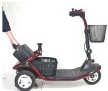
Figure 14. Removing the Battery Pack
