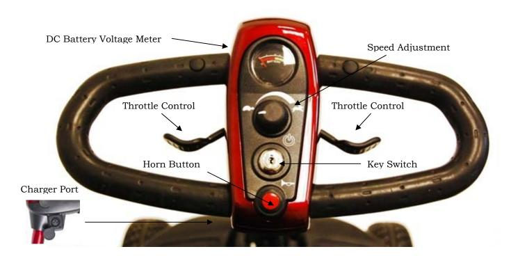
Figure 5. LiteRider<sup>TM</sup> Delta Tiller Control Panel
