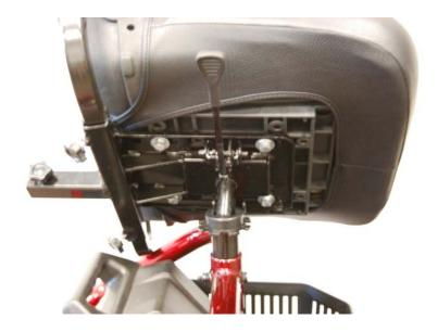
Figure 23. Installing the Seat
