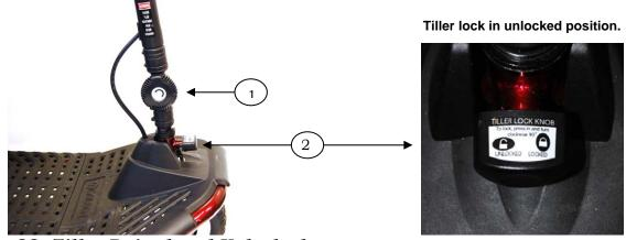
Figure 22. Tiller Raised and Unlocked
