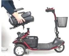
Figure 13. Removing the Seat
