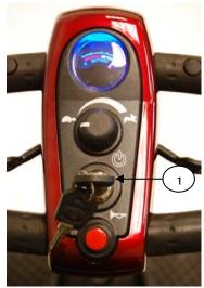
Figure 12. Key Switch (On)
