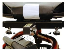
Figure 6. Armrest Width Adjustment
