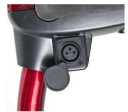
Figure 25. Charging Batteries
