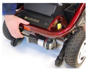
Figure 17. Releasing the Drivetrain
