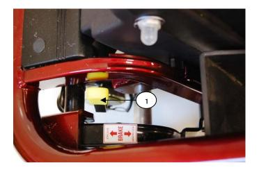
Figure 9. Freewheel Mode (Brake Disengaged)
