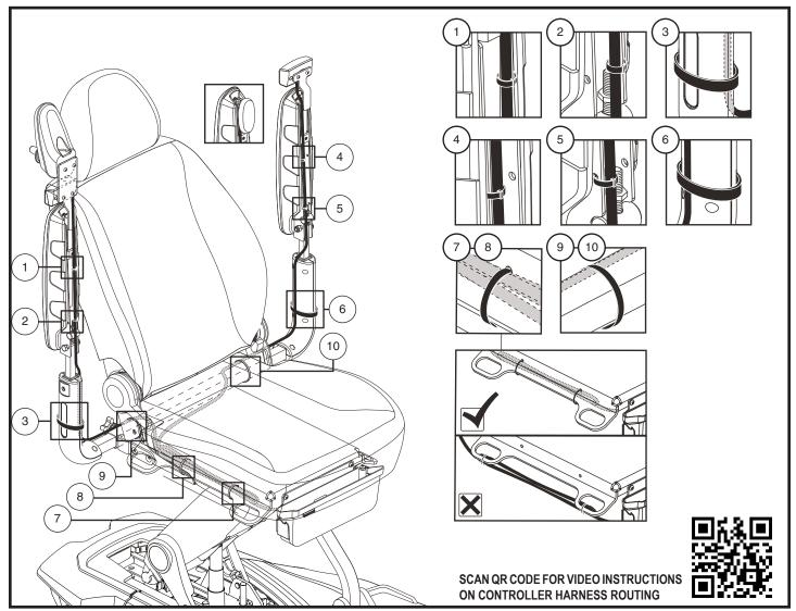
Figure 11. Controller Harness Routing
