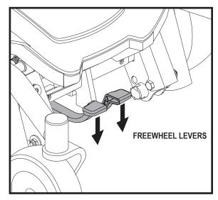
Figure 5. Freewheel Mode (Drive Disengaged)
