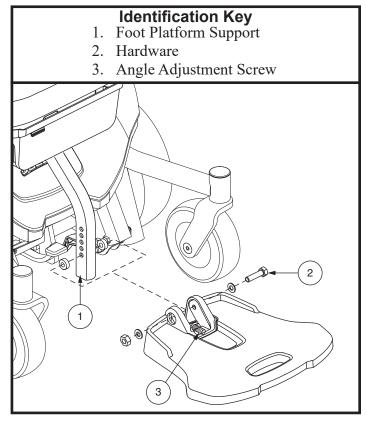
Figure 13. Foot Platform Adjustment
