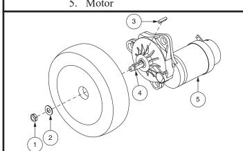
Figure 16. Drive Wheel Removal
