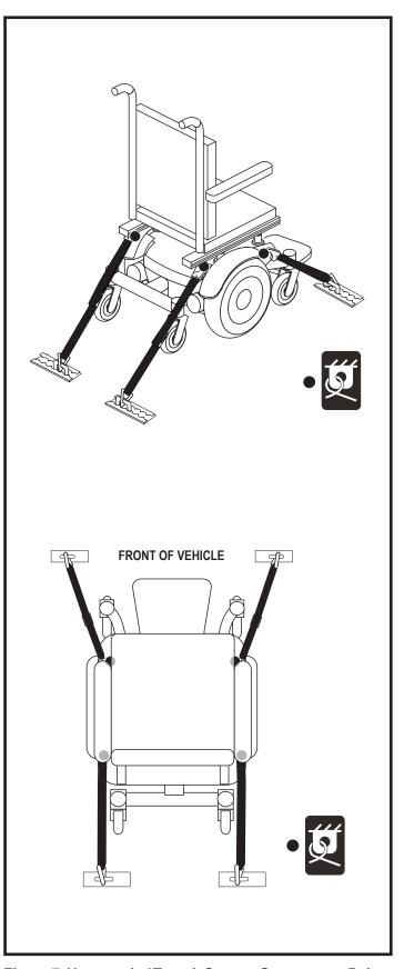
Figure 7. Unoccupied Transit System Securement Points
