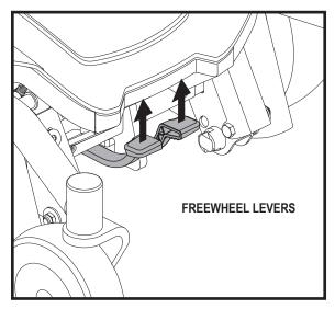
Figure 4. Drive Mode (Drive Engaged)
