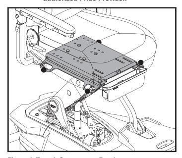
**Figure 6. Transit Securement Brackets**
