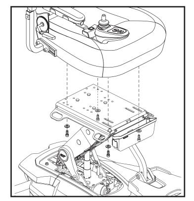
Figure 10. Seat Installation
